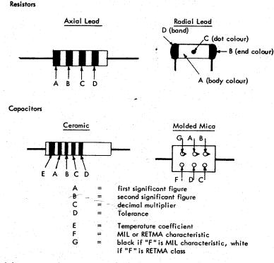
Figure 1.1 Arrangement of Component Colour Coding
